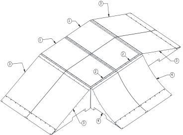
• Connect upper surfaces of the concrete elements by using sheet metal connectors (point 7,8 and 9) and countersunk screws of point 15.
