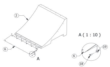
Screw the steel toe plates (point 7) to the Banks (point 1) by using screws and washers of point 14, 18 i 19.
