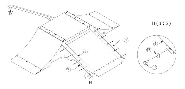
Install the side rails (point 10, 11, 12, 13) with the screws and washers of point 18 and 19.
