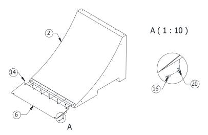
Screw the steel toe plates (point 7) to the Banks (point 3) with screws and washers of point 14, 16 and 20.
