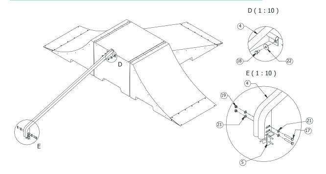
Install the side rails (point 9, 10, 11, 12, 13) by using screw and washer of point 16, 20.
