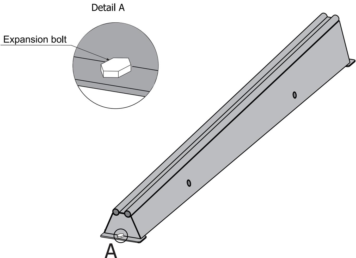
Figure 1. Assembly scheme
