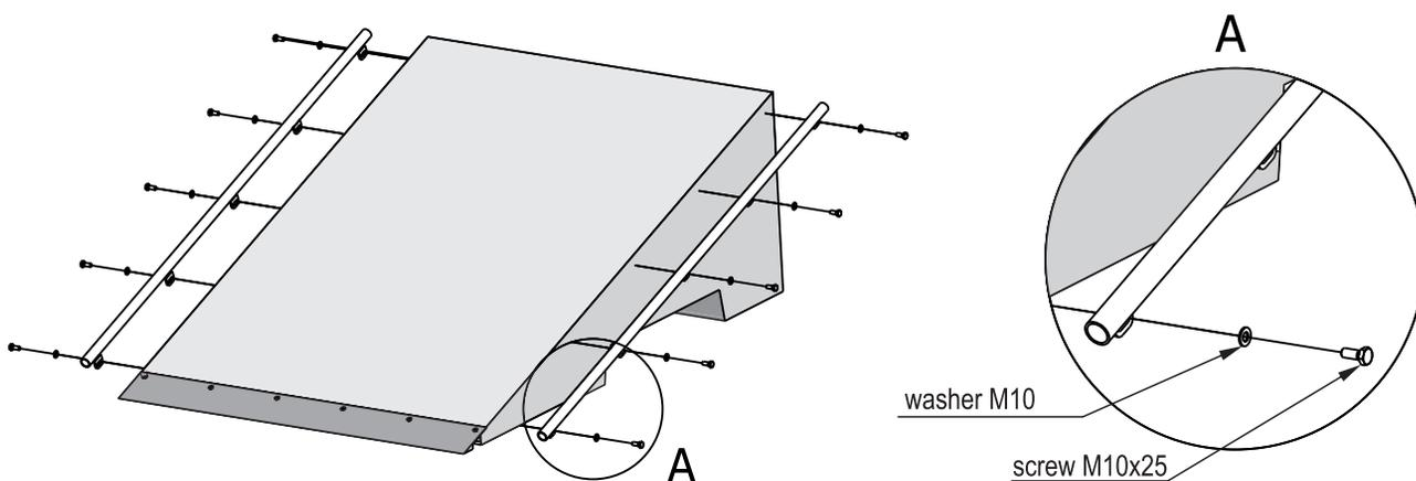
Rys. 2 Assembly of the side rails.
