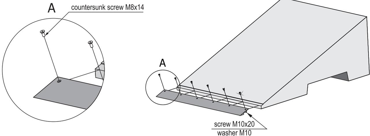
Fig. 1. Steel toe plates assembly method
