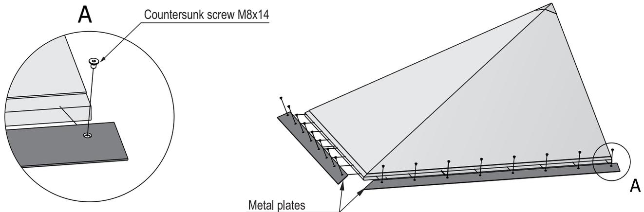
Rys. 1. Metal plates assembly method
