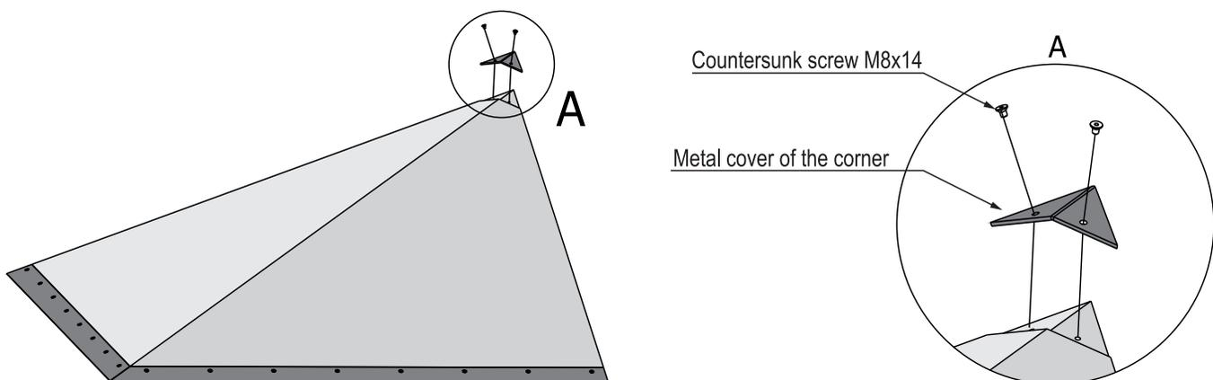
Rys. 2. Metal cover of the corner assembly method.
