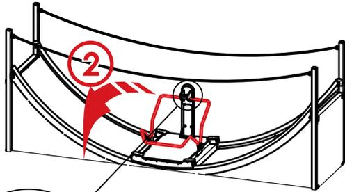
① Release the barrier of the platform by moving the safety lock
