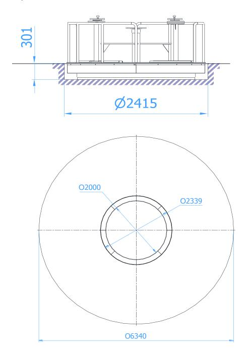
WARNING ! All installation activities shall be performed in accordance with health and safety standards A foundation setup tolerance is  $\pm$  50 mm.
