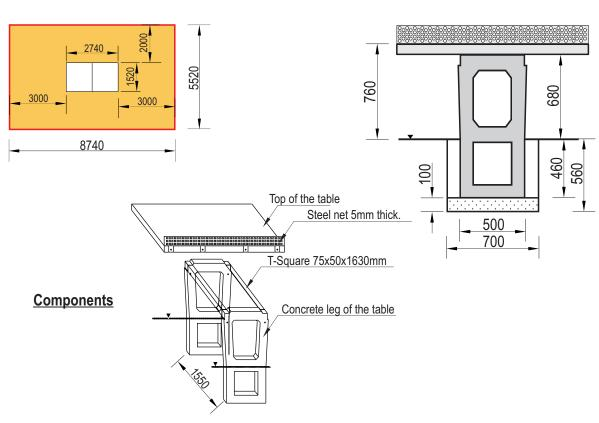
3. Assembly works shall be started by screwing two table legs with two T-squares 75x50x1630mm by using M10 screws.
