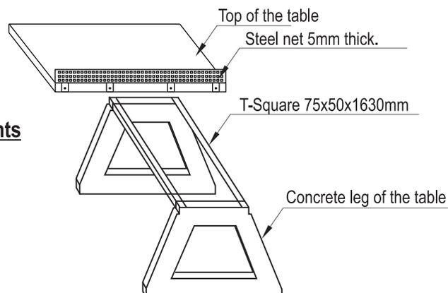
3. Put the with T-squares 75x50x1630mm on the table legs and screw it by using M10 bolts.
