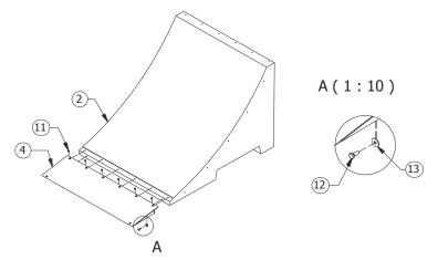
Screw the steel toe plates (point 5) To the Banks (point 3) by using screws and washers of point 11, 12 and 13.
