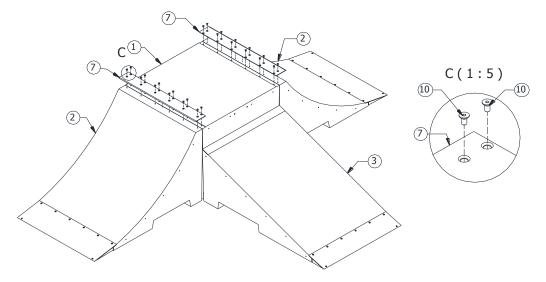
• Screw the side rails (point 6, 8, 9, ) by using screws and washers of point 12 and 13.
